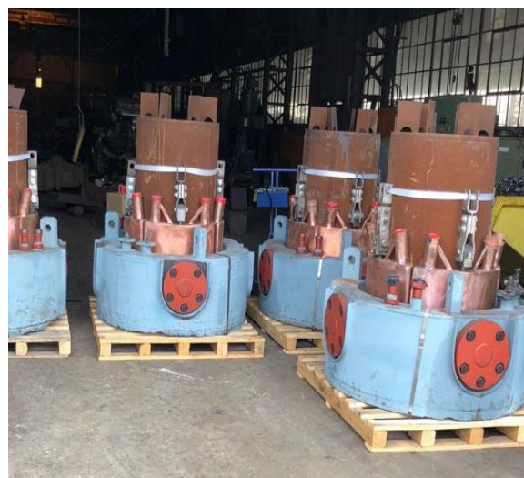
Figure 4: Lower Electrode Copper Contact Shoes and Stainless Steel Pressure Ring on pallets, ready for shipping
