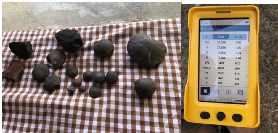
Figure 5.2 – Manganese Nodules Samples and XRF Reading (Mn 58%)
